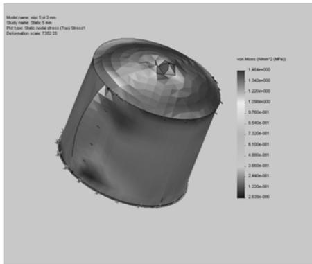
**Fig. 11.** Maximum mechanical tension after Von Mises stress theory
