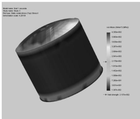
**Fig. 7.** Maximum mechanical tension after Von Mises stress theory
