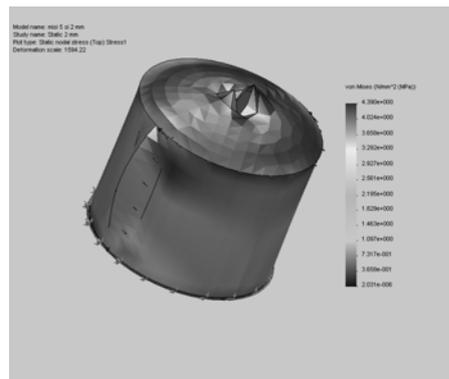
**Fig. 14.** Maximum stress after Von Mises stress theory
