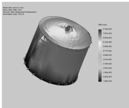
**Fig. 13.** Maximum deformation occurs in the middle of the tank
